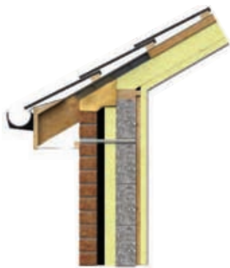
Partial Fill Cavity Wall
