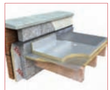
Typical installation - Timber Deck
